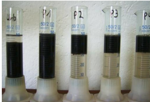
Figure 12: Floating up of sludge irradiated with 800 W
