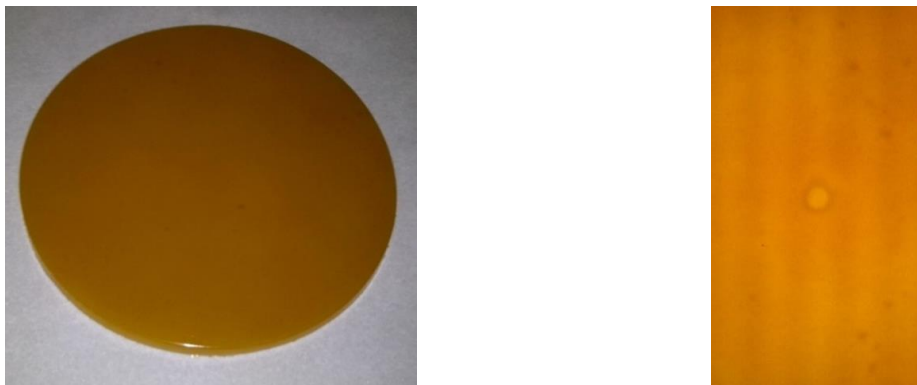
Obr. 3.7 Model S5 - dutina v izolante (detail)
