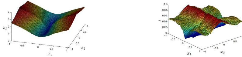
Obr. 2.12: CSR model. On the left, energy function E(i_1, i_2, 50) for a mesh 100 \times 100 \times 100 with chosen x_3 in the middle of region of interest. On the right, error estimation for mesh 100 \times 100 \times 100 with chosen x_3 in the middle of region of interest.
