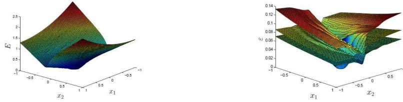
Obr. 2.8: Inverted Pendulum. On the left, energy function E(i_1, i_2) for a mesh 100x100. On the right, error estimation for meshes 100x100, 75x75, 50x50 from bottom to top. Error estimation decreases with increasing mesh size.
