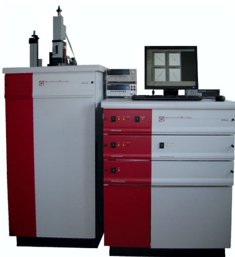
Obr. 3.1 SQUID magnetometer/susceptometer MPMS XL-7 od firmy Quantum Design.
