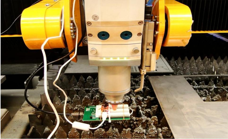
**Figure 5.5:** The STM32F3DISCOVERY board mounting for acceleration measurements
