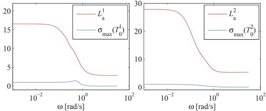
Figure 3: Verification of the robust stability condition in each mode (2.23)
