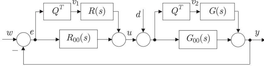
Figure 1: Switching feedback loop
