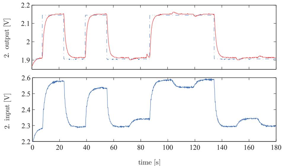
Figure 18: Measured reference, second input and second output signal during experiment
