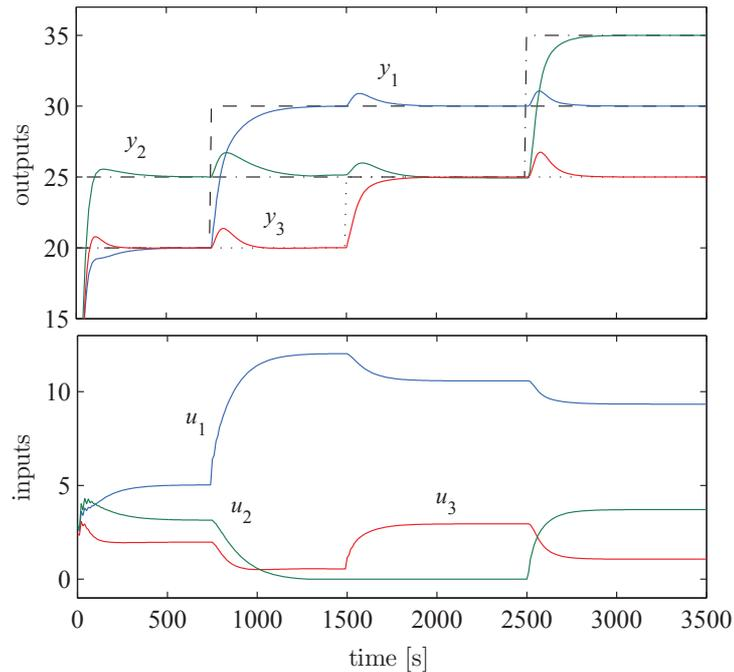
Figure 9: Time responses of the system inputs, outputs and set-points
