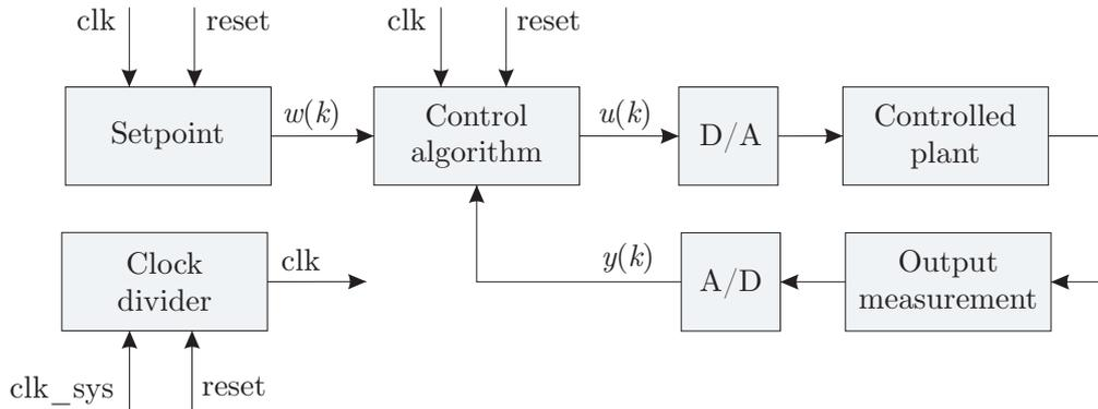
Figure 11: Control loop block scheme
