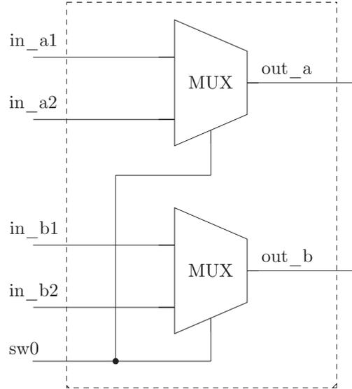
Figure 12: Switch implementation scheme
