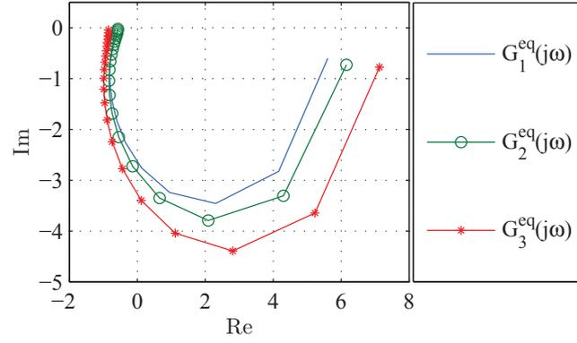
Figure 8: Nyquist frequency response of equivalent subsystems for selected  $g_2(z)$
