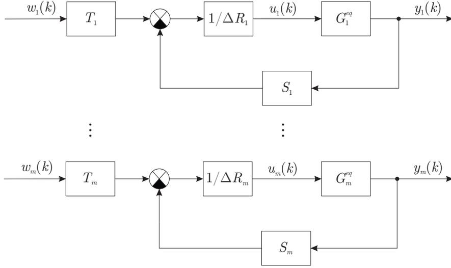
Figure 7: Polynomial structure of the decentralized controller for MIMO system represented by equivalent subsystems
