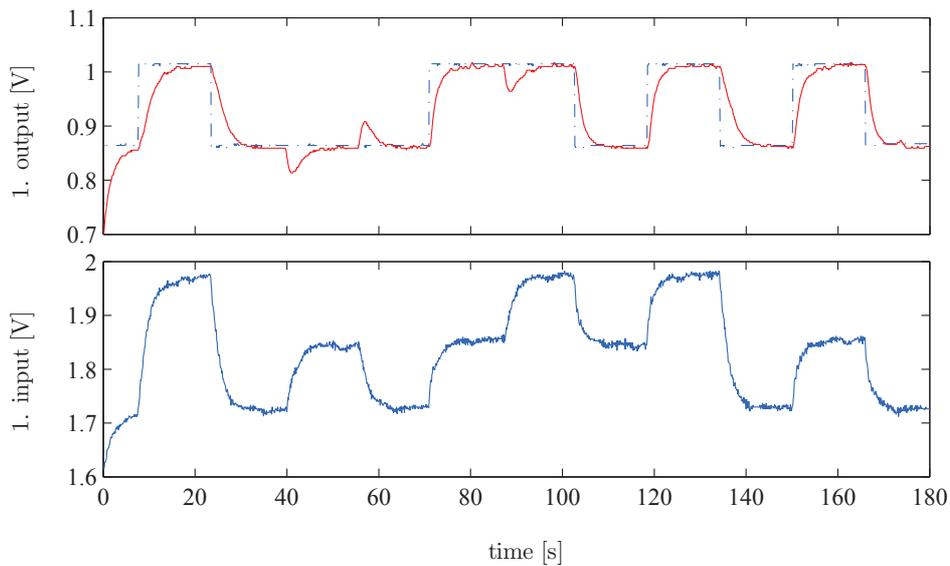
Figure 17: Measured reference, first input and first output signal during experiment
