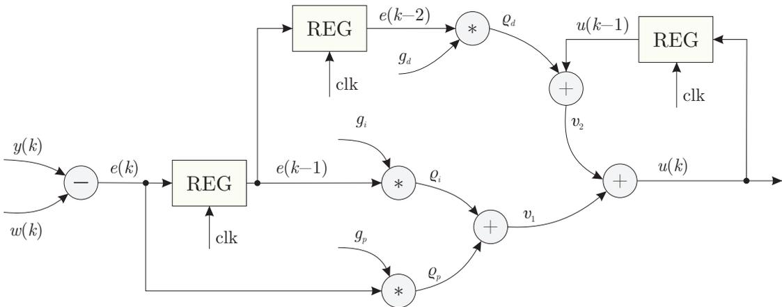
Figure 10: Parallel design of incremental PID algorithm
