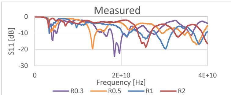
**Fig. 5** Measurement of the return loss parameter for loop inductor designs. (Credit: Asoc. Prof. Martin Tomáška, PhD.)
