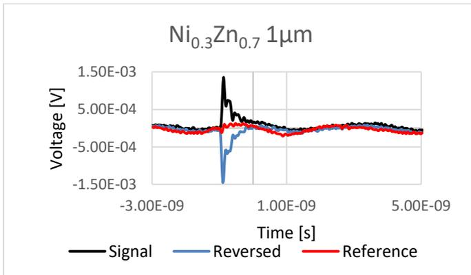
**Fig. 6** Characteristics measured using a 1 micron thick sputtered Ni<sub>0.3</sub>Zn<sub>0.7</sub>Fe<sub>2</sub>O<sub>4</sub> layer with the loop diameter of 2 mm under applied external magnetic field (signal), without external magnetic field (reference) and with the external field direction reversed (reversed).
