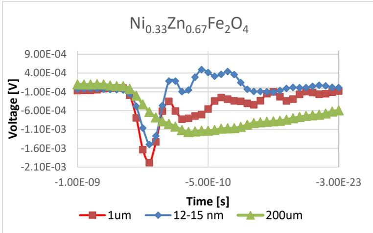
**Fig. 7** A comparison of rise times of demagnetization induced signals from  $\text{Ni}_{0.33}\text{Zn}_{0.67}\text{Fe}_2\text{O}_4$  powder sample with 200  $\mu\text{m}$  grain size, 1  $\mu\text{m}$  and 12-15 nm sputtered layer using a 1 mm diameter inductor.
