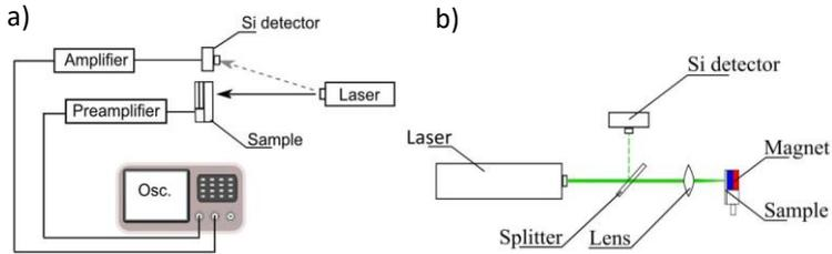
**Fig. 3** Block scheme of the measurement setup (a) and the optical setup layout (b)
