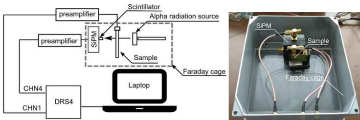
**Fig. 8** A schematics (left) and actual (right) layout of the experimental set-up, used in alpha particle induced thermomagnetic effect experiments.
