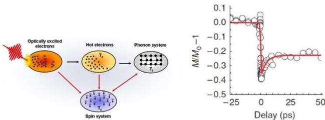
**Fig. 1** A graphical representation of the three temperature model, where  $T_e$  is electron temperature,  $T_s$  spin system temperature and  $T_l$  lattice temperature and an actual demagnetization characteristic of a CoPd multilayer film [8].
