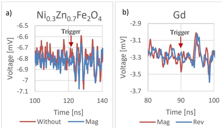
**Fig. 9** Measured and averaged characteristic of 1  $\mu\text{m}$   $\text{Ni}_{0.3}\text{Zn}_{0.7}\text{Fe}_2\text{O}_4$  ferrite deposited on 12  $\mu\text{m}$  PEN without applied magnetic field (red) and with applied field (blue) (a) and a plasma etched Gadolinium membrane with applied field (red) and field direction reversed (blue) (b).
