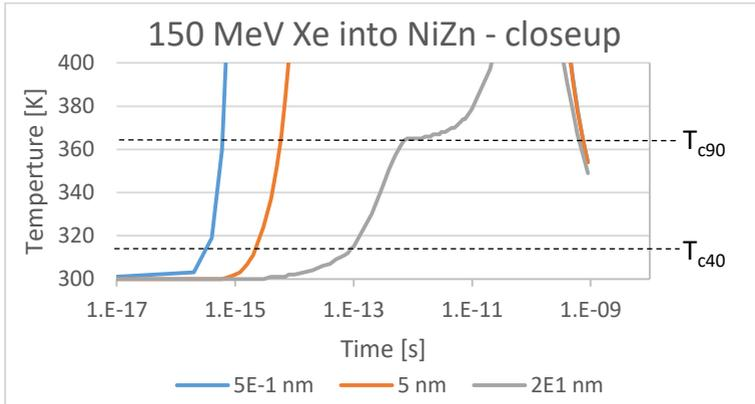
**Fig. 2** Thermal spike simulation of a 150 MeV Xe ion in NiZn ferrite with lines representing curie temperatures of 40 ( $T_{c40}$ ) and 90°C ( $T_{c90}$ ) is shown in the figure for 0.5, 5 and 20 nm radius around the particle track.
