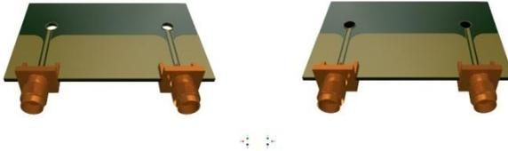
**Fig. 4** 3D view of the second generation of loop antenna designs, where a design of a 1mm diameter loop antenna with a hole (right) and without hole (left) is shown.
