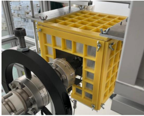
Figure 19: The KOSTKA device installed around the experimental chamber [22].
